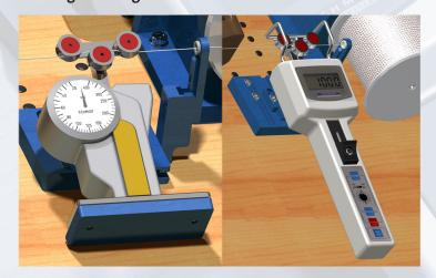
The Tension Meter with data memory and interface enables an optimal tension adjustment and facilitates statistical analyses.
