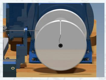
Equipped with a slot for yarn clamping.
