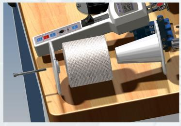
The conical shape of the wind up spool makes it easy to remove filling yarn.
