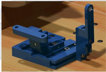
The Tension meter support is constructed specially to enable an exact position adjustment of the gauge rollers to the filling yarn at different shuttle variations. Furthermore the position of the ceramic guide eyelet is also exactly adjustable to the filling yarn.
