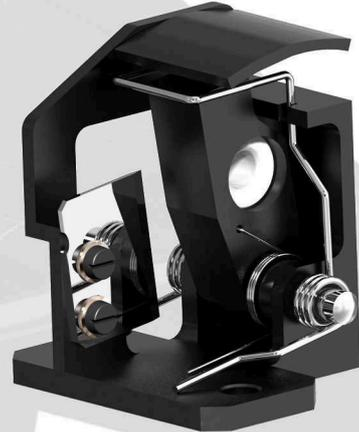
Modular yarn cutter type B "left version", made of black anodized aluminum with integrated yarn cutting equipment. The yarn guide is ensured by a polished ceramic eyelet.
