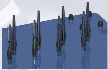
The arrangement of the pirn spindles as well as of the yarn brakes and ceramic eyelets has been designed accordingly the seam fabric weaving process. 4 BCF-Single Yarns are positioned on the left side of the seam cable and further 4 BCF-Single Yarns on the right side. This configuration enables the formation of a better seam reinforcement at the tissue side as well as at the loop side.
