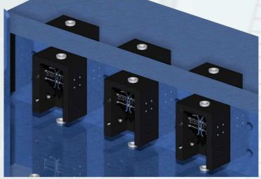
The ceramic eyelets order at the fastening bracket is equivalent with the positioning of the seam cable bobbin and the pirn arrangement at the unit. A crossover of the yarns could not take place.
